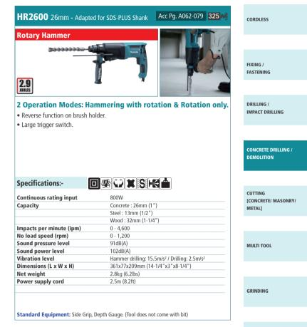
Standard Equipment: Side Handle, Depth Gauge. (Tool does not come with bit)
